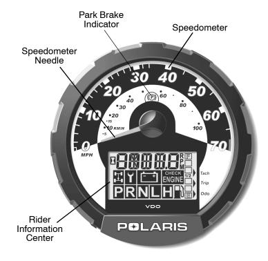
**NOTE:** In addition to showing vehicle speed, the speedometer needle flashes when a low fuel condition exists.
